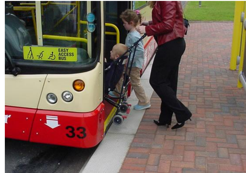
Picture 4-8: Standard Curb Bus Boarding
