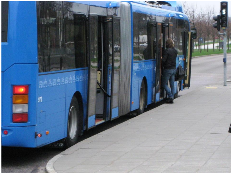
Picture 4-9: Raised Curb Bus Boarding, Rapid Bus, Goteborg, Sweden
